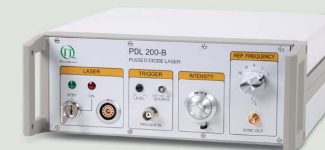
As an alternative to the PDL 800-B/D, the PDL 200-B is available. This driver has five fixed internal, user-selectable repetition rates of 8, 4, 2, 1 and 0.5 MHz. It can also drive all laser heads of the LDH-P Series as well as all LEDs of the PLS Series.
