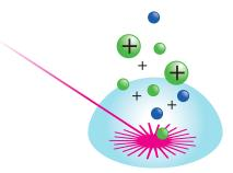
**DNA IONIZATION:** The analyte crystals are irradiated by a laser, inducing desorption and ionization of the molecules
