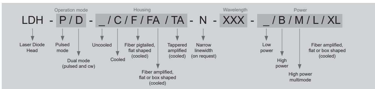
C: Laser head with thermoelectric cooler, mandatory for some laser heads, optional for all other laser heads
