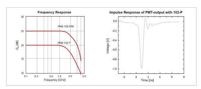
The PAM 102 pre-amplifier is specially targeted at timing sensitive applications such as Time-Correlated Single Photon Counting (TCSPC) with fast photon detectors like Microchannel Plate PMTs (MCP) or standard PMTs. Such detectors produce very small output pulses with extremely short pulse widths, usually too small for direct interfacing with TCSPC electronics or other counters.
