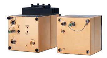
The PMA detector is a single photon sensitive, fully integrated, fast time response and low noise photon sensor from Pico-Quant. The PMA integrates a fast Photomultiplier Tube (PMT), a high voltage power supply and pre-amplifier. For selected models thermo-electric cooling and automatic overload protection are available as an option.
